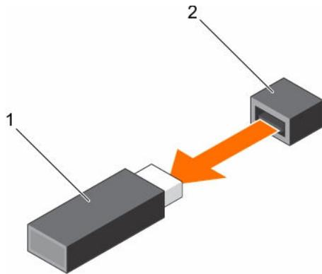
**Figure 47. Removing the internal USB key**
