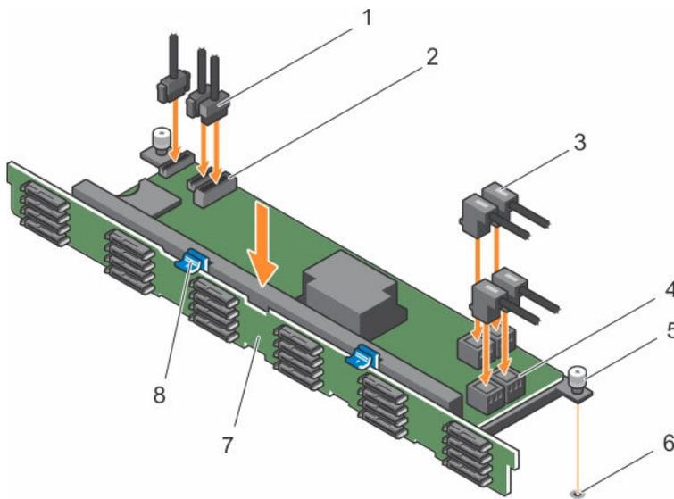
**Figure 88. Installing the 1.8-inch (x24) hard drive backplane**
