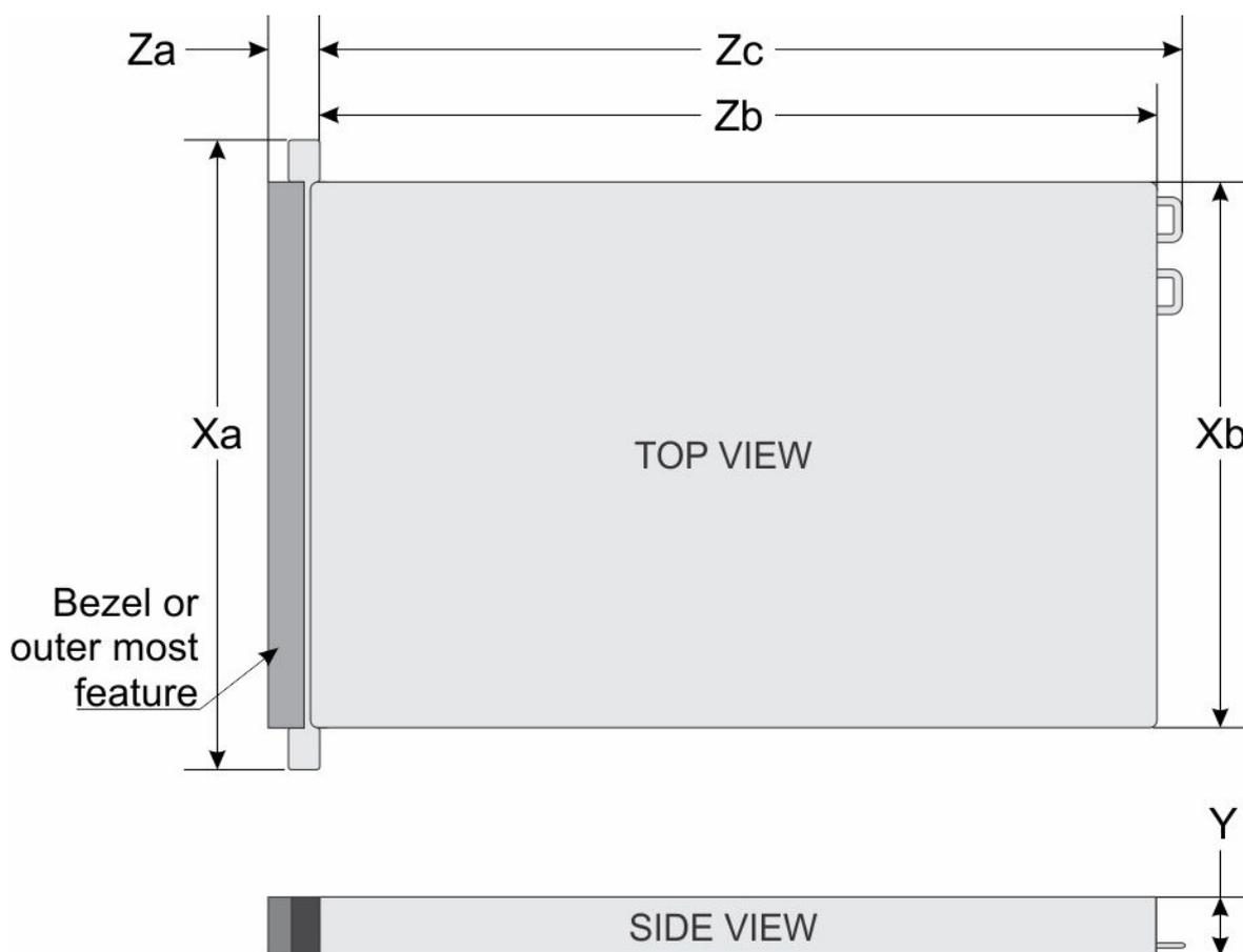
Figure 15. Chassis dimensions of PowerEdge R630 system
