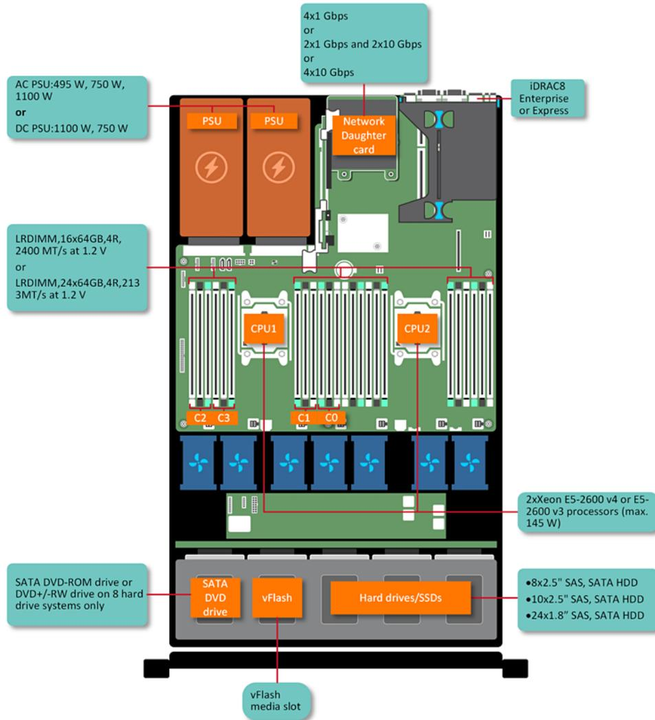
Figure 1. Supported configurations for the PowerEdge R630 system
