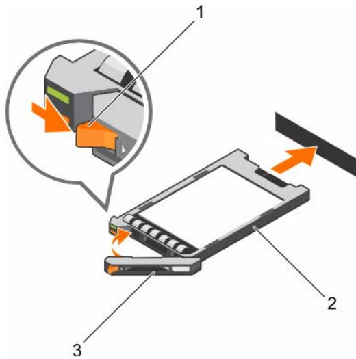
**Figure 36. Installing a 1.8-inch hot swappable uSATA SSD**
