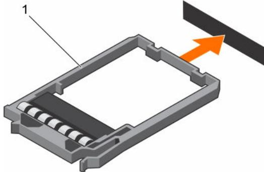
Figure 32. Installing a 1.8-inch hard drive blank
