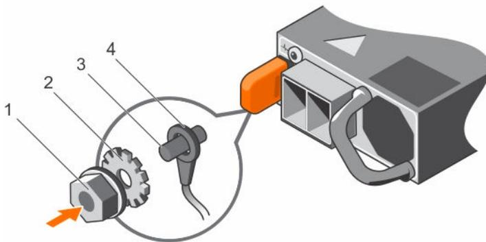
**Figure 72. Assembling and connecting the safety ground wire**
