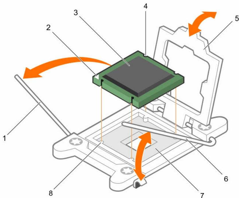
**Figure 65. Removing and installing a processor**
