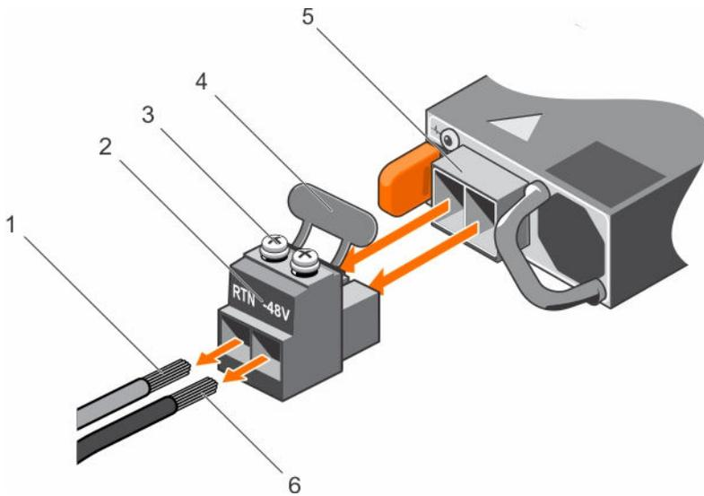
**Figure 75. Removing the DC Input Power Wires**
