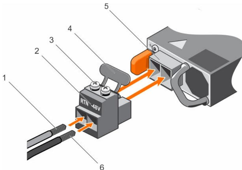
Figure 74. Assembling the DC Input Power Wires
