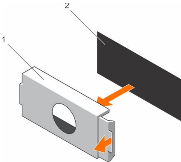
**Figure 68. Removing the PSU blank**
