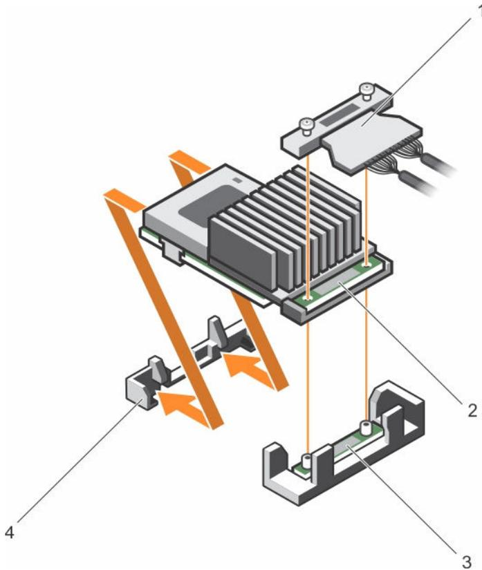
**Figure 60. Installing the integrated storage controller card**
