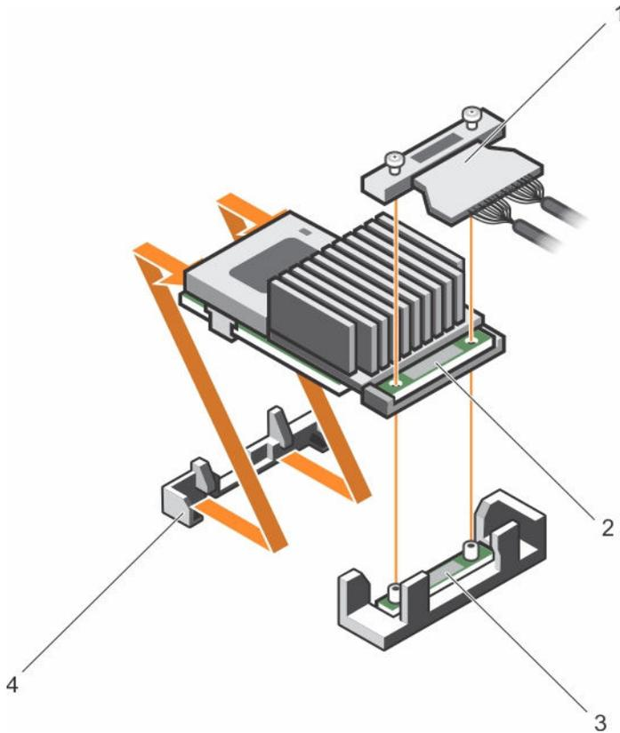
**Figure 59. Removing the integrated storage controller card**
