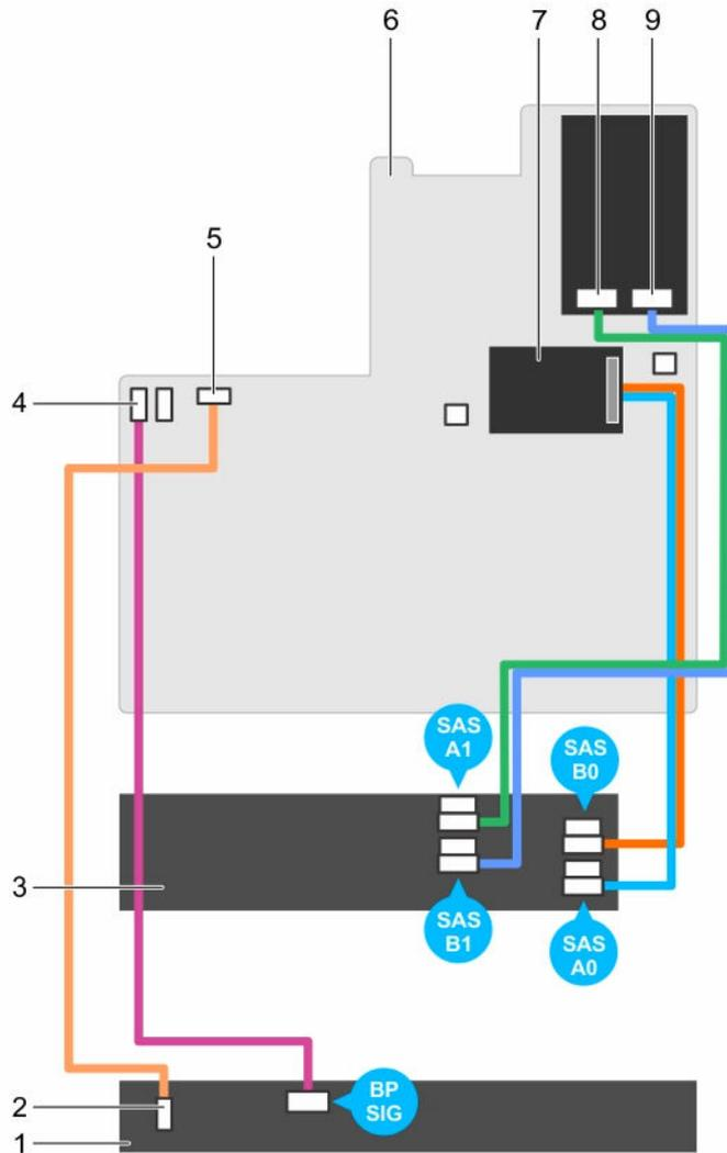
**Figure 85. Cabling diagram—1.8-inch (x24) hard drive systems**
