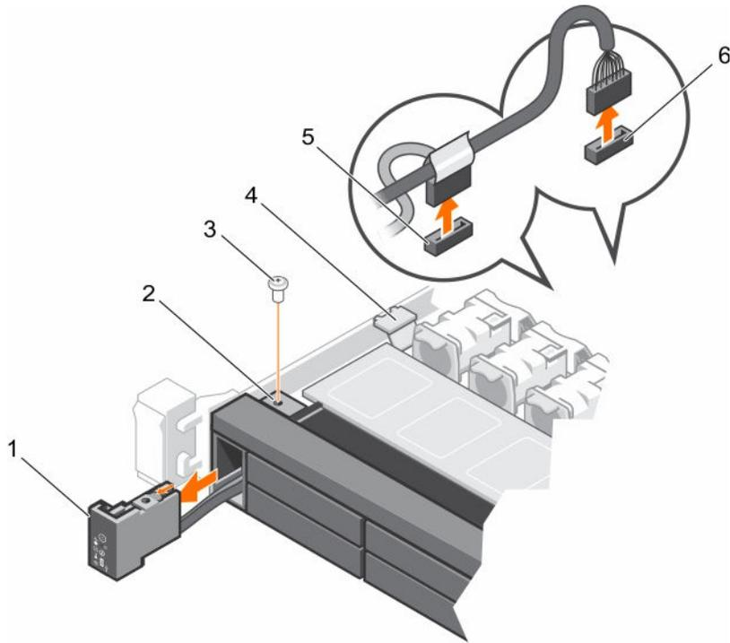
**Figure 93. Removing the control panel for 10 and 24 hard drive system**
