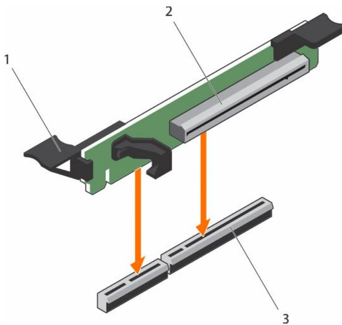
**Figure 54. Installing the expansion card riser 3**
