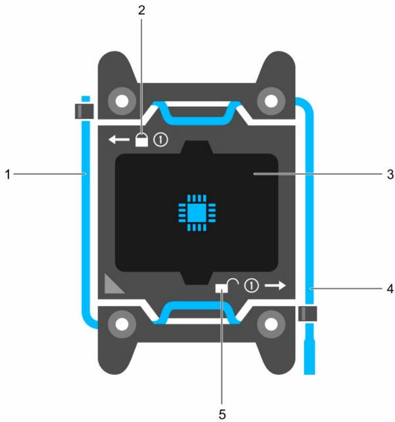
**Figure 64. Processor shield**
