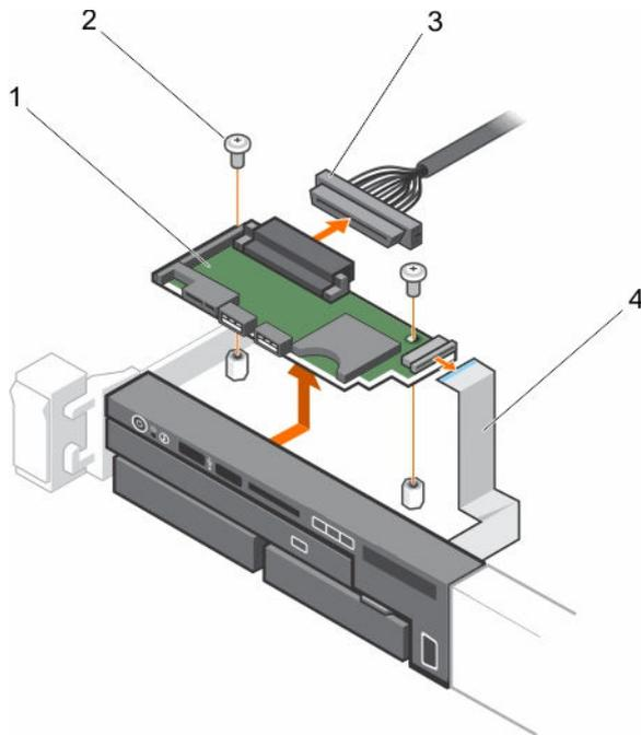
**Figure 89. Removing the control panel board**
