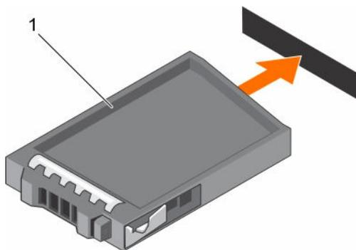
**Figure 30. Installing a 2.5-inch hard drive blank**
