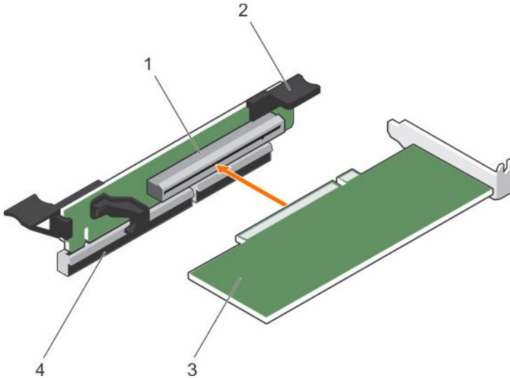
**Figure 52. Installing an expansion card**
