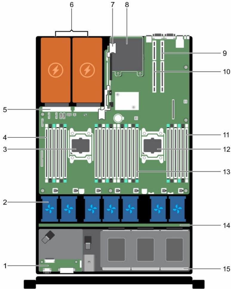
**Figure 22. Inside the system—eight hard drive system**
