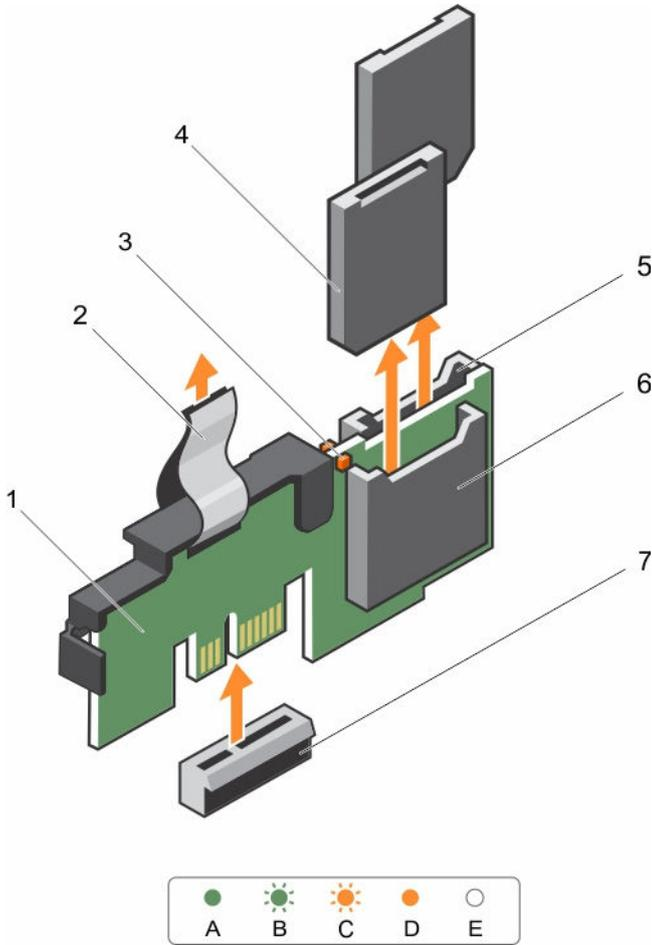
**Figure 57. Removing the internal dual SD module (IDSMD)**
