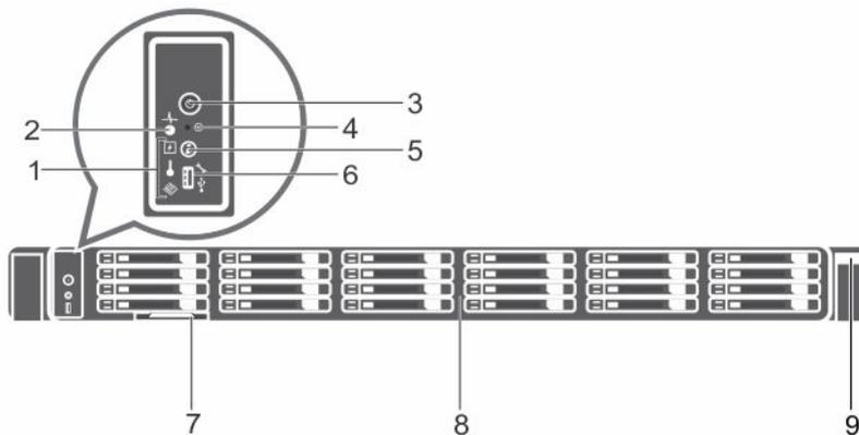
**Figure 4. Front panel features of the 24 x 1.8-inch hard drive PowerEdge R630 chassis**
