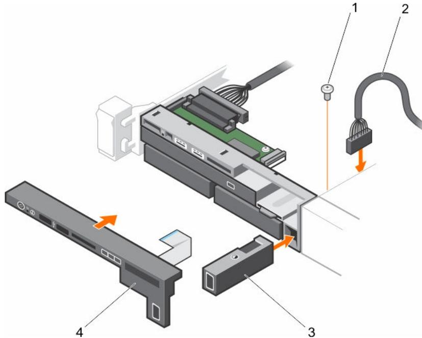
Figure 96. Installing the VGA module
