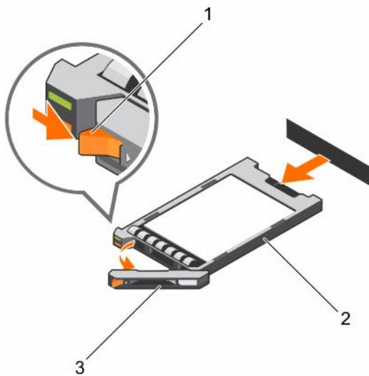
**Figure 34. Removing a 1.8 inch hot-swappable uSATA SSD carrier**
