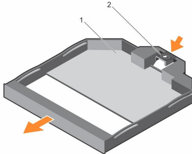
**Figure 43. Removing the slim optical drive blank**
