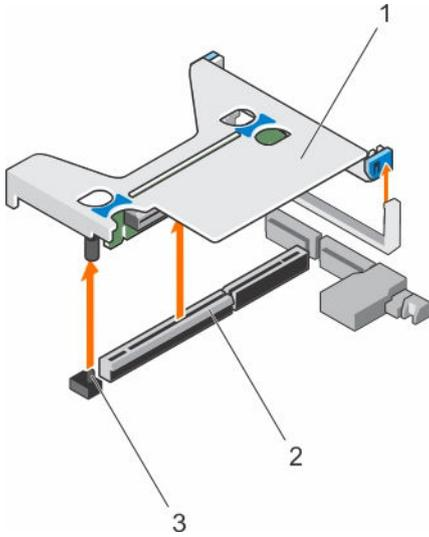
**Figure 49. Removing the expansion card riser 1**
