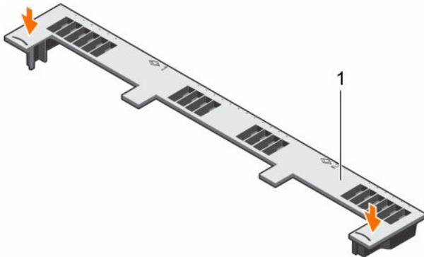
Figure 25. Installing the cooling shroud
