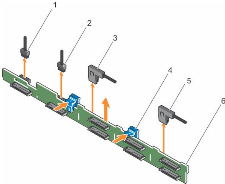
**Figure 80. Removing the 2.5-inch (x8) hard drive backplane**
