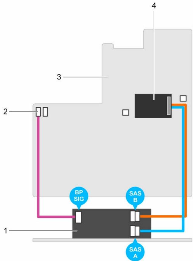
**Figure 83. Cabling diagram—2.5-inch (x10) hard drive systems**
